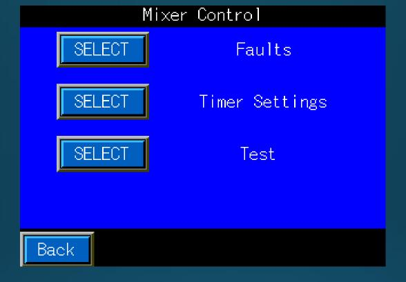
Mixer Control Menu, press SELECT to navigate to the required screen or Back to return to the previous screen
