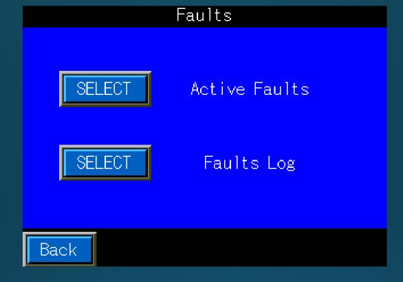
Faults Menu, press SELECT to navigate to the required screen or Back to return to the previous screen
