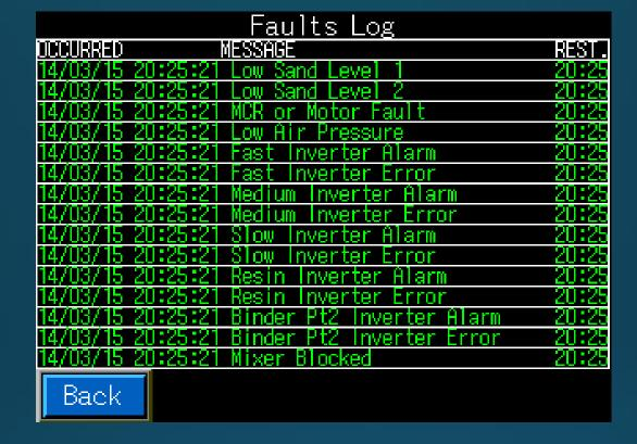
• Faults Log, this displays the status of the system, anything with errors will display in yellow, when displayed in green the faults is cleared, also displays the time the fault was cleared
