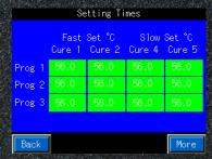
Setting times offset temperature to speed up or slow down cure times.
