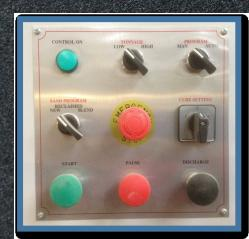
An operator panel connected at the front of the mixer contains the controls for; Start, Pause & Discharge, it also contains an emergency stop, sand programme selection that suits the customer requirements, 5 set time selection switch giving you; very fast, fast, normal, slow and very slow cure times, auto or manual blend switch, this allows temperature to control cure time
