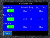
Temperature probe calibration, gives better control of temperature settings. (IBS ONLY)
