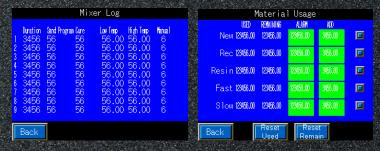
Mixer run duration, sand program, cure setting, temperature and manual program log.
