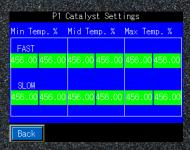
Catalyst temperature settings, enter min, mid and max temperature.
